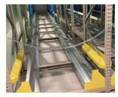
◆ Capacity of 12 pallets per lane Each lane can store 12 pallets deep. When a pallet is placed in the front, the shuttle automatically carries the products to the back. This equipment is well suited for storing products in large lots.
