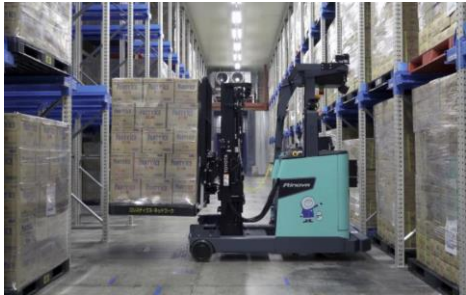
Verification tests begun for automated forklift operations in the harsh work environment (-25℃) inside refrigerated warehouses
