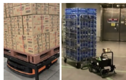
AGV for transporting pallets
