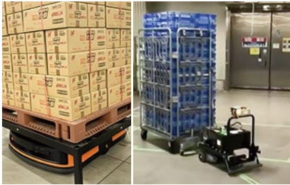
AGV for transporting pallets AGV for transporting roll pallets
