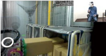
Robot operator using goggles to check the cockpit view for remote control operation
