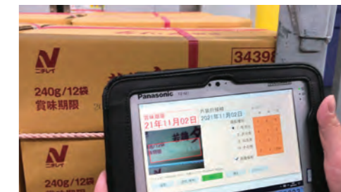
* Automated expiration date reader AI solution: AI-OCR (Optical Character Recognition/Reader) recognizes images using image preprocessing technology to identify the characters of the expiration date from the image and match the recognized expiration date with information in the cloud, to enable more accurate readings.
